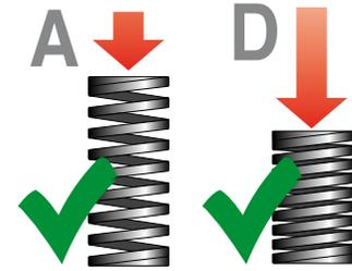
**EN** If the measurements of the spring constant is made with deflections below the values stated in column A, or with deflections over the values stated in column D, the results obtained can be out of the tolerance of +/- 10% on the nominal value.
