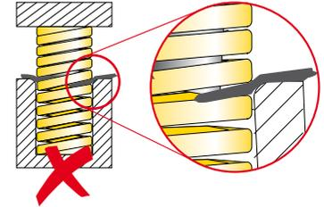
**EN** Any alteration on the surface of the springs (cutting, grinding, scratching, etc.) may significantly reduce the lifetime. Always replace damaged springs with new ones.
