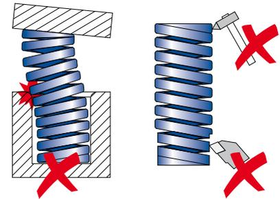
**EN** If one spring collapses, an imbalanced load will occur with possible subsequent damage to the other springs. Replace all springs as a set. Advance planned maintenance prevents damages and saves money.
