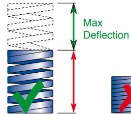
**EN** The greater the pre-load the longer the lifetime for the same total deflection. Thus, longer springs with same total force, will assure longer lifetime. It is recommended to always apply a minimum pre-load of 5% of the free length. Absent or insufficient pre-load causes unexpected failure to the springs.
