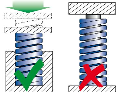
**EN** Proper guiding is essential to long life. It is recommended to always guide springs with a free length /diameter ratio exceeding 3.5.
