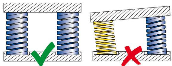
**EN** Tool maintenance (grinding, die sharpening) can vary the original working deflection of the springs because of the subsequent decrease in shut height. Always check and re-set the original working stroke. Failure to respect this requirement may result in high risk of early failures or damages to the tool.
