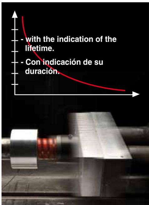
**EN** Ongoing in-house reliability tests allow Special Springs to provide estimated service life values of springs in compliance of working deflections and recommendations. The stated service life values are not guaranteed due to the impossibility to consider all variables on the real working conditions of the springs.
