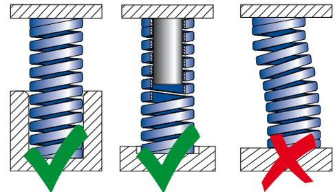
**EN** Avoid the use of insufficiently guided, stacked springs or nested springs due to high risk of serious damage and injury.
