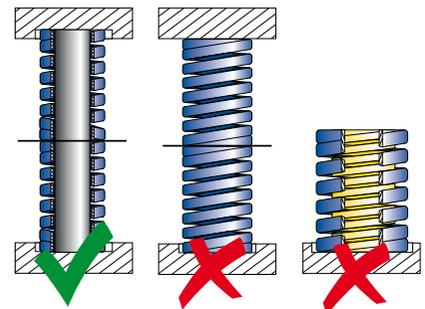
**EN** When using different types of springs simultaneously, ensure that deflections and forces guarantee a balanced load. Always ensure the best perpendicularity between surfaces to avoid early failure of the springs.
