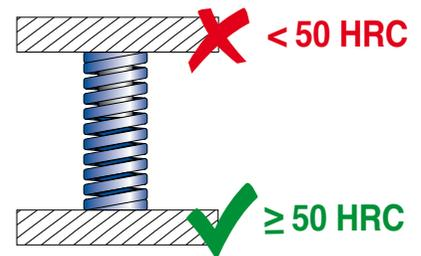
**EN** Do not apply forces other than in the compression direction. Using compression springs as extension or torsion springs will cause deformation and sudden failure. The improper use of springs may bring unforeseen accidents with damage and injury.
