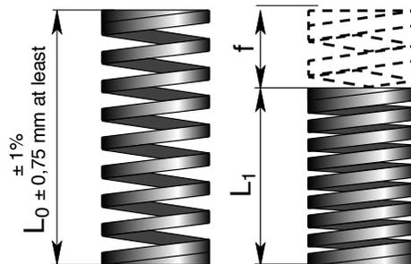
**EN** For a better understanding, the example below shows the calculation of the nominal value of force and the min and max values possible for the spring RHL 125-300 at a given length L<sub>1</sub> of 55,1 mm - 2.17 inch as follows:
